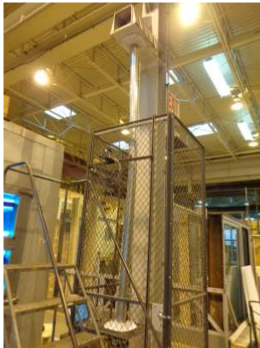
Photo No. 2 Typical Axial Load Compression Test Setup (120 in length post)
