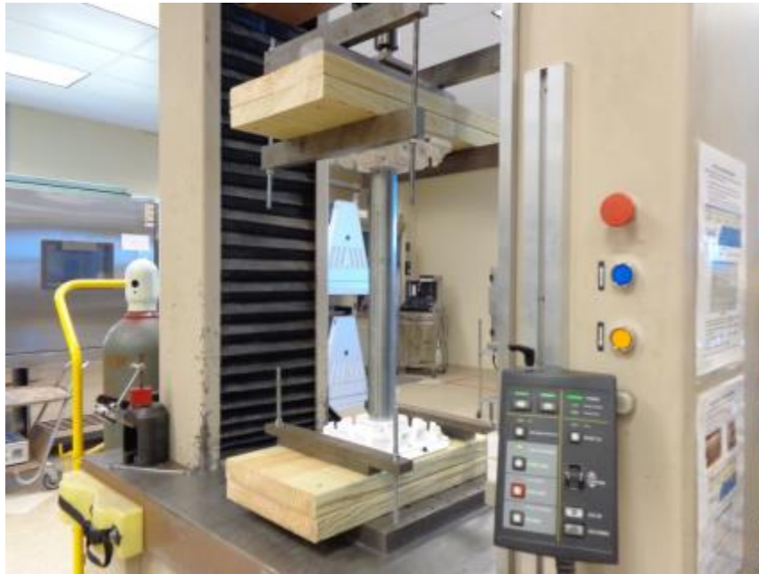
Photo No. 3 Typical Uplift Load Test Setup
