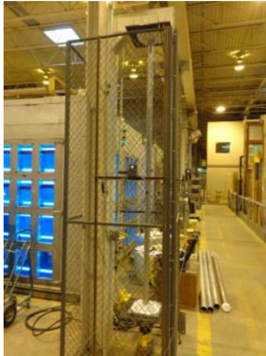
Photo No. 1 Typical Axial Load Compression Test Setup (108 in length post)
