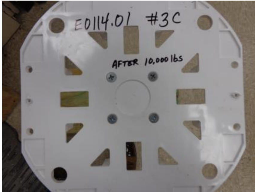
Photo No. 9 Punching Shear Test Results Following 10000 lbs of Load - 2-3/8 in Diameter Post (Specimen 3 - Underside)
