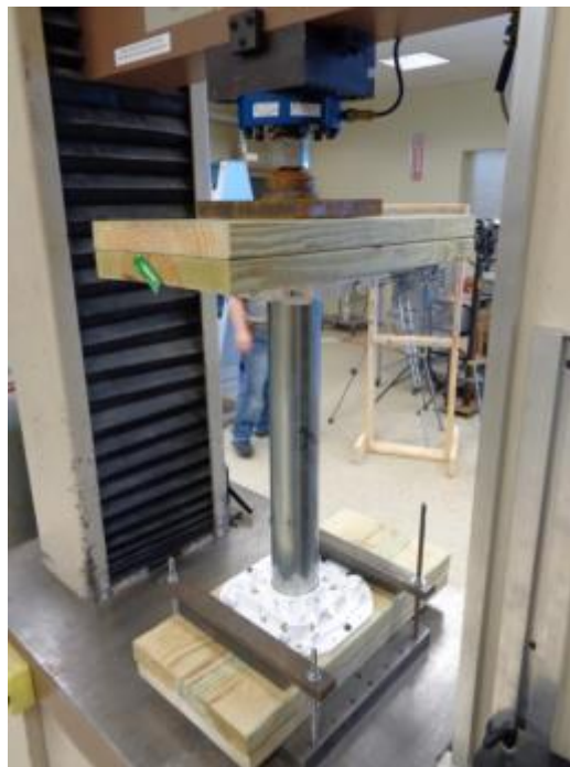
Photo No. 6 Typical Punching Shear Test Setup
