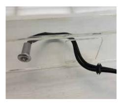
**4. Grommet Replacement**Pull the wires out through the routed holes next to the 11/32" hole.
