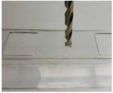
**1. Drill**Drill a 11/32" hole for inserting the LED light flush to the rail.
