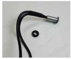
**2. Grommet**Remove the grommet completely from the wires.
