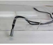
**3. Slide** Slide wires through 11/32" hole pushing the LED light flush.
